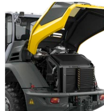
Optimal service accesses: The WL95 and WL110 offer easy-to-access maintenance flaps and the mudguards can be removed. This allows easy access to the engine, hydraulic system, and electronics. This greatly facilitates the inspection and maintenance of the machine. The engine hood can be opened widely, thereby allowing for optimal access.
