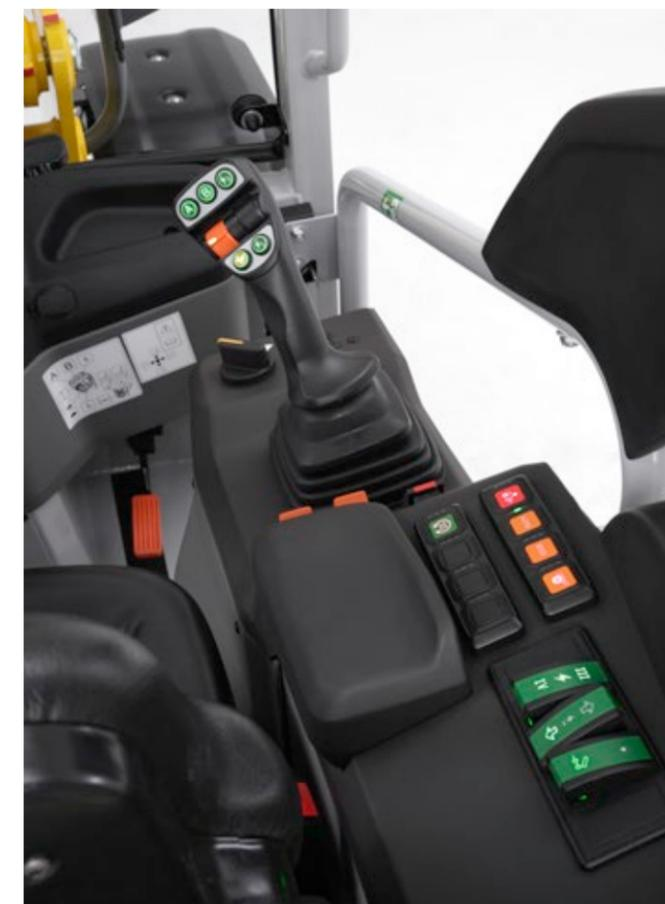
Drive smarter with the WL28. The electronically controlled travel drive ensures extremely high driving comfort and increases the machine's thrusting force. In addition, various travel modes are available.
