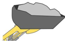
The maximum possible bucket capacity is determined via the tipping load and the payload:
