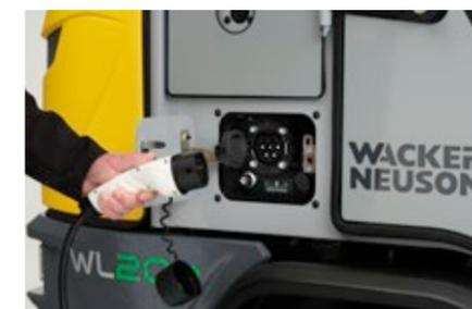
2. Open charging cover, insert Type 2 plug on the machine.
