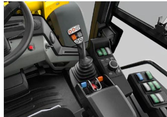
Hydraulic oil volume adjustment easily via "Jog Dial": If an attachment does not require the full hydraulic performance, the flow volume can be reduced manually. In this way, the operator can work sensitively with the machine and attachment while saving resources.
