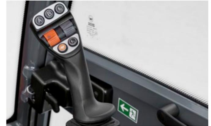
Operator-friendly and multifunctional: the innovative joystick with ergonomically-arranged, illuminated touch keys.
