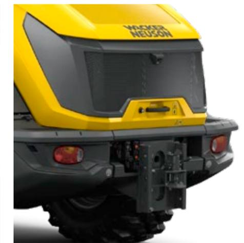
Trailer operation up to 18 tons: WL95 and WL110 have a self-recovery coupling as standard. In addition, the following coupling possibilities are available: automatic ball hitch, K50 ball hitch (car trailer), Auto Hitch, Piton Fix, as well as CUNA D3. To safely move trailer loads, there is both a two-line pneumatic brake as well as a hydraulic trailer brake.
