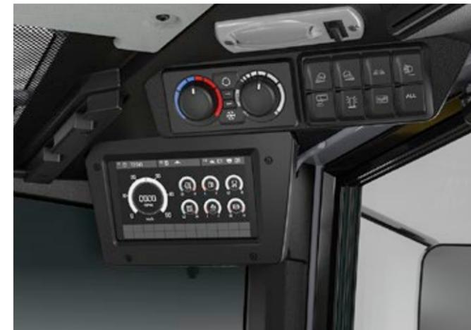
With a digital 7"-display, keep everything in view: In addition to the standard displays, such as the temperature, tank fill-level and operating hours, active functions are displayed in the cockpit, such as active electrical functions, the continuous operation of the 3rd control circuit, or the activated differential lock.
