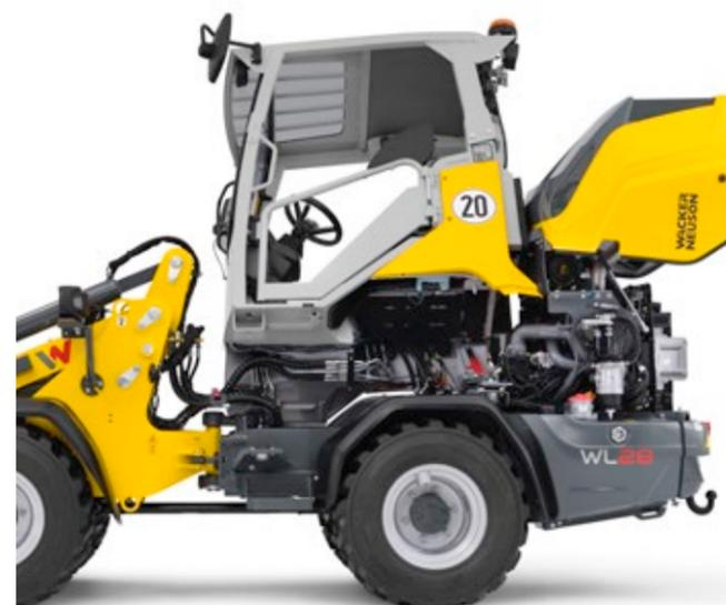
All three wheel loaders are outfitted with a tiltable operator's cab or a fold-down cabin. This allows easy access to the engine, hydraulic system, and electronics. The engine hood can be opened widely, thereby allowing for optimal access.
