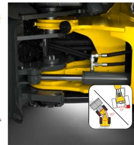
Rear articulated joint and oscillating axle: Tight curves, small slopes – every construction site is different. In order to bring the transported material safely to the destination, the WL95 and the WL110 are equipped with an articulated joint and an oscillating axle in the rear. This ensures the optimum maneuverability and traction in any situation. At 40°, the steering angle is generous, the turning circle over tires is 4.90 m and the inner radius is 2.45 m.
